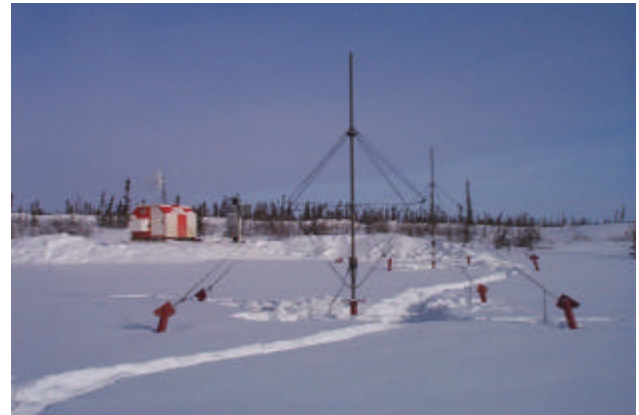
Figure 7: Fixed Receive Antenna
